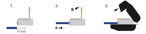
**1.** Strip the wires according to the specified dimension of the corresponding splicing connector and Inline Splicing connectors with lever series 221.
